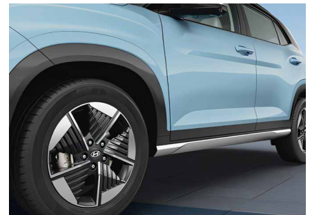
R17 (D=436.6 mm) Aero alloy wheels with Low Rolling Resistance (LRR) tyres
